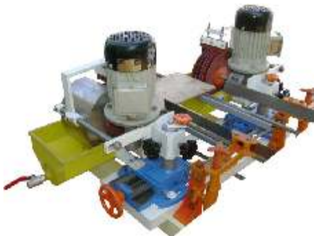
Water Scrapping Device Suitable for removing excess glaze from tile sides
